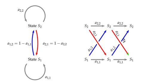
Markov model on states: limited lookback (horizon) :  $p(X_{t+1} = s_i | X_1 \dots X_t) = p(X_{t+1} = s_i | X_t)$  (1) Stationary $p(X_{t+1} = s_i | X_t) = p(X_2 = s_j | X_1)$  (2) Transition matrix: $a_{ij} =$  (3)
