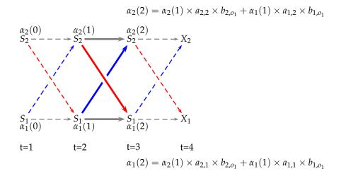
Let's calculate the probability of being at state *i* at time *t*, after emitting t-1 letters. This amounts to summing over all the paths only the first part of the path-string probability. That sum of products is the *forward* quantity  $\alpha$ . The part that is left over (the sum over all the path-strings to the right of *t*) will be summarized with the *backward* quantity  $\beta$ .
