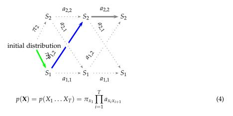
The probability of taking a path *X* and generating a string O is equal to the product of the probability of the path times the probability of emitting the correct letter at each point on the path.
